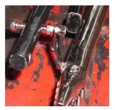
The cylinder head nuts have a very uncommon 9mm X 1.25 thread pitch. Once again, these nuts had to be made from 14 mm 316 stainless steel hex stock and then nickel plated.
