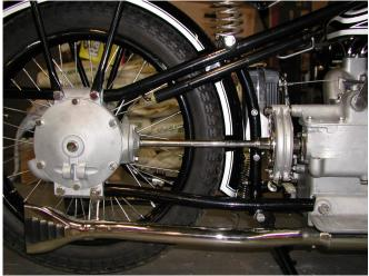
While I looked for a correct rear brake and driveshaft, I continued to use the incorrect R11 parts. About this time, I should mention that most of the nuts bolts and hardware on this series of motorcycle are unique to these machines. These are just a few of the nuts and bolts that I made for the R62 and the World's Best R12. All of the mounting hardware on the R62 is finished with nickel plate.
