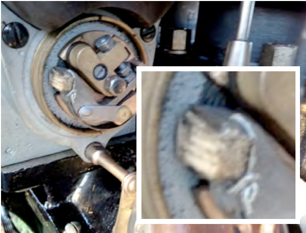
My wooden rubbing block repair.
