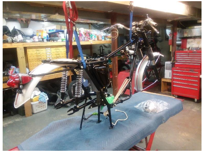
More fender fitting and wiring mock-up.
