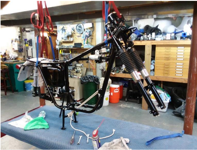
Fender fitting and wiring mock-up.
