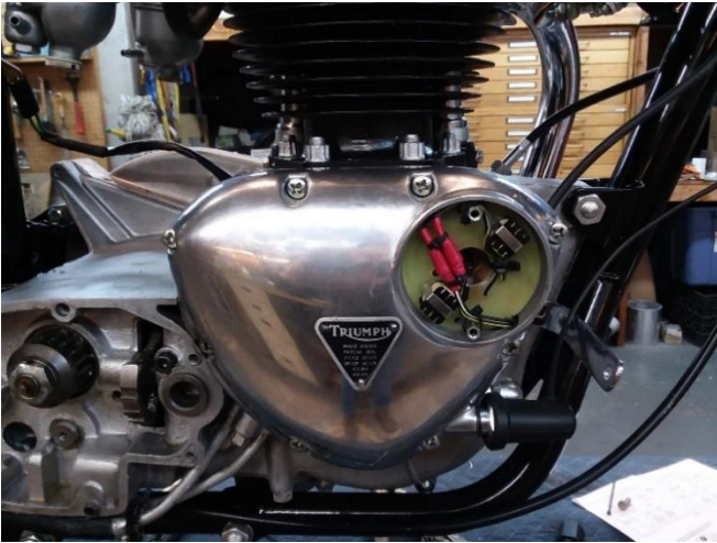
New points plate replacement.
